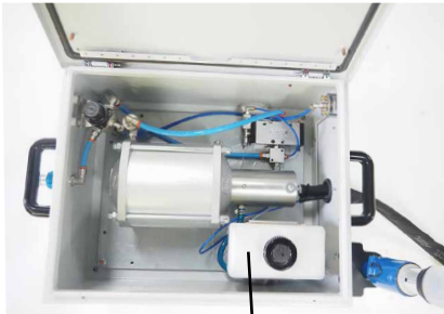
*Tank locked, remove safety lock.
